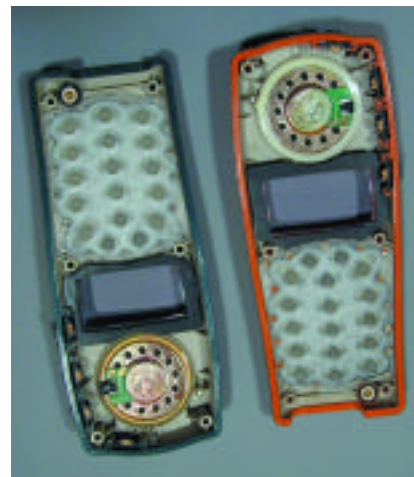
Inside view of ruggedized GSM radio front cover. Note four custom designed snap dome pogo pin switches, used to interface to integrally molded rubber keys. The design facilitates Z-axis assembly while providing an extremely rugged and watertight enclosure.
