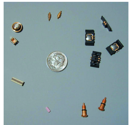
Advanced interconnect technology components developed for the Ericsson, Inc. GSM rugged radio. Clockwise from top: Double acting pogo pins for speaker, pogo pin snap dome switches for front cover side and top rubber keys, internally/externally sealed pogo pin screws for the battery connection, elastomeric connector for the microphone, elastomeric connector for the LCD, and injection molded/formed metal contact connector and pogo pin connector for the system and remote antenna interfaces, respectively.
