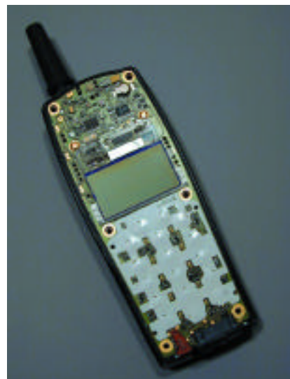
PCB and rear cover subassembly of GSM radio. Note LCD lightguide with integrally molded speaker pogo pin and LCD elastomeric connector captivation geometry (upper left and upper center, respectively, of lightguide). Directly above the lightguide are the two sealed screw/pogo pin battery interconnects. At the lower left corner of the PCB is the microphone elastomeric connector and molded housing.
