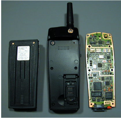
Ruggedized GSM radio battery, rear cover assembly and PCB. The injection molded/formed metal system antenna connector is in the upper right corner of the PCB. The pogo pin remote antenna connector is in the upper right corner of the rear cover assembly. Also visible are the two sealed pogo pins for the battery contacts (directly below the remote antenna connector). The mating battery contacts are shown on the adjacent battery.
