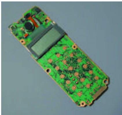
Populated PCB of a push to talk (PTT) radio developed in the mid nineties. Note the use of heat seal connector and flex/ZIF connector at the LCD. Additionally, there is an elastomeric connector at the upper left hand corner of the PCB, which is used to terminate a front cover mounted microphone. Thus we see new interconnect technology beginning to mingle with the old.
