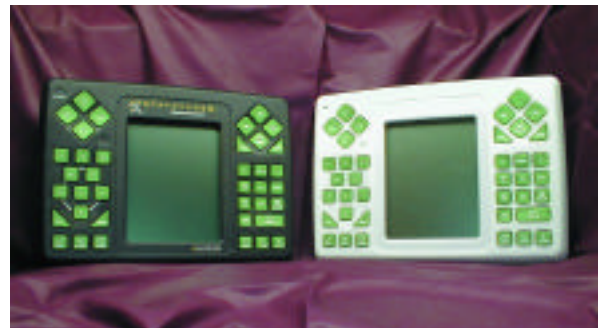
A select group of U.S. product design companies are using in-house prototyping to support increasingly aggressive and cost efficient product development schedules. The proof of concept model on the right was generated in a fused deposition modeling (FDM) prototyping system, while a production unit is depicted on the left.
